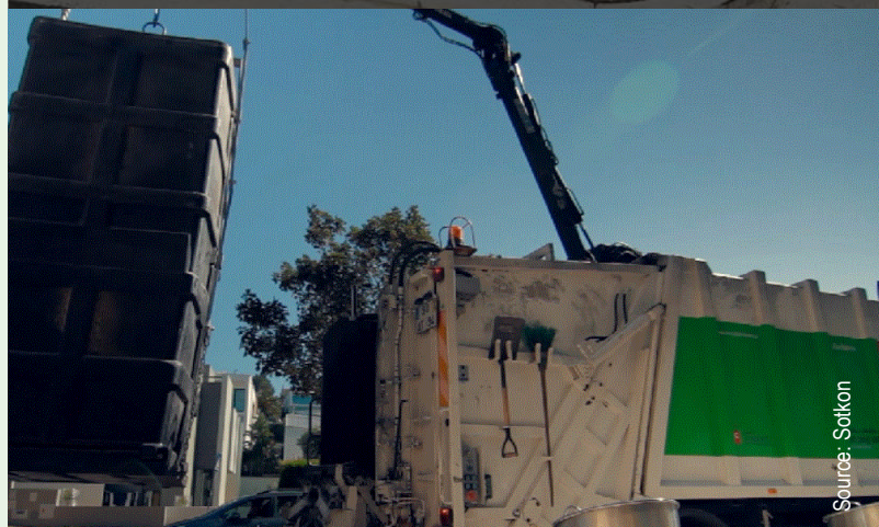
Crane-lift Truck for Single Bin Units, Portugal
